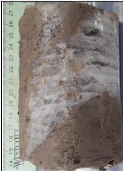
Figure 5. Segregated ice lens in clayey silt core sample, Yellowknife region.
